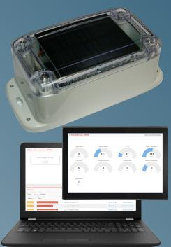
Nexcomm System's TrackPoint Mobile is a small, cellular gateway designed for outdoor tracking and sensing applications. It uses an integrated GNSS receiver and reports its location through a CAT-M1 cellular modem. Dallas 1-Wire and one input give it the ability to connect to sensors for real-time monitoring of equipment.
