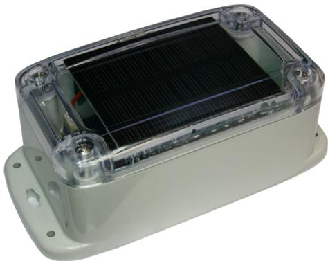
The TrackPoint Mobile is a small discreet mobile tracker that reports its GPS location on a configurable interval. It has a motion sensor that allows it to sleep until it detects movement. This allows it to last for up to three years on a D-cell primary battery or longer on a solar rechargeable 18650 battery.
