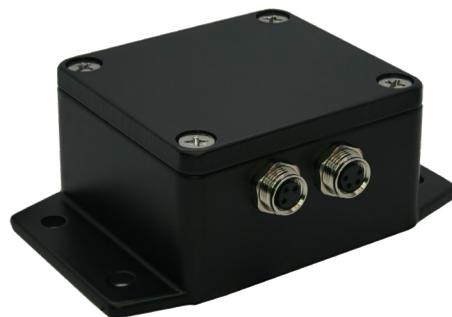
The SensePoint Serial node has one RS-485 and one RS-232 channel for communication to controllers, PLCs, or sensors. It communicates with a Nexus gateway over a Wi-Fi HaLow or customized Thread wireless link. This allows serial commands and data to be passed from a cloud server to the connected device through the Nexus system.
