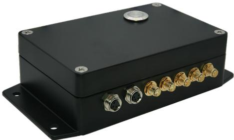
The Nexus Industrial gateway communicates with SensePoint nodes over Wi-Fi HaLow or a customized Thread wireless network. It uses a CAT-1 cellular modem to communicate with cloud servers.
