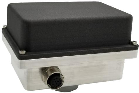
The SensePoint Accel node includes a three-axis accelerometer for vibration measurements in Condition Based Monitoring (CbM) applications. With a 6kHz bandwidth and 16g dynamic range, the SensePoint Accel is suitable for monitoring for bearing faults as well as imbalance and misalignment.
