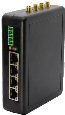
The Nexus Panel gateway is designed in a DIN rail enclosure for mounting in any standard control panel. With one USB channel and one RS-485 channel, it can easily interface to a wide range of PLCs, motor controllers and pump controllers. A digital input can be used as an alarm or trigger and a digital output can
