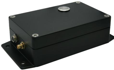
The SensePoint Motor node has three 1V CT channels and eight PT100 RTD channels. It is designed to verify the health of electric motors by monitoring the motor currents and temperatures of various components. It communicates with a Nexus gateway over a Wi-Fi HaLow or customized Thread wireless link.
