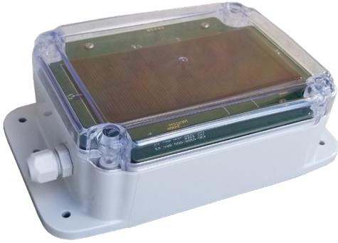
The EdgePoint RTU is a generic hub for monitoring and control. It can control solenoids and valves for irrigation, agriculture and pumping applications. It can interface to a wide array of sensors for monitoring anything from HVAC systems to landfills and waterways. An integrated solar power option makes the
