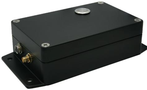
The SensePoint Industrial node offers 4 channels of 4-20mA analog inputs, 4 channels of 0-24V analog inputs and four channels that are 0-48V digital inputs. A single Dallas 1-Wire channel enables operation with digital sensors. A 50V power input makes it compatible with 48V industrial systems. It communicates with a Nexus
